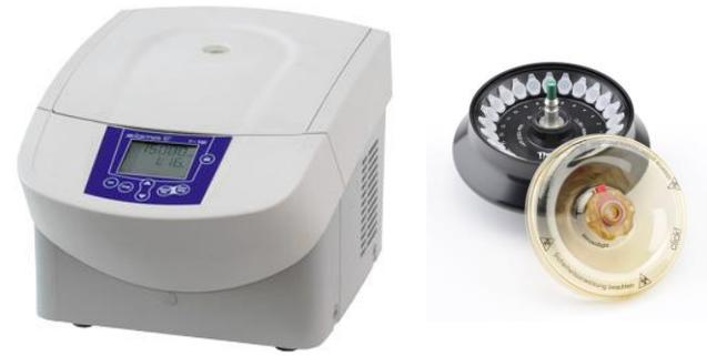
Centrifuge spins tubes at 14,000 revolutions per minute (rpm) for 2 minutes
